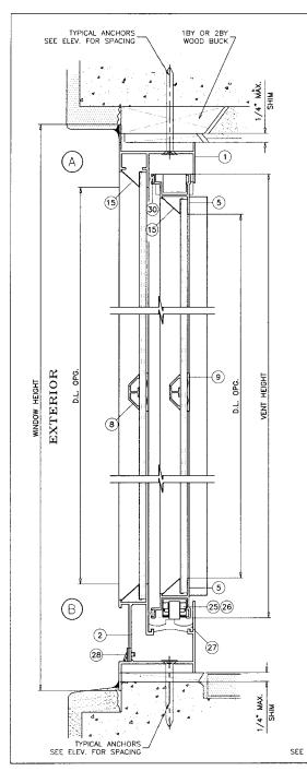
METAL FL # 0027689 (STEEL OR ALUM, 1/8" MIN. THICK) STEEL: Fy = 36 KSI MIN. ALUMINUM : 6063-T5 MIN.
