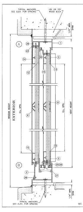
METAL FL # 0027689 (STEEL OR "ALUM. 1/8" MIN. THICK) STEEL: Fy = 36 KSI MIN.
