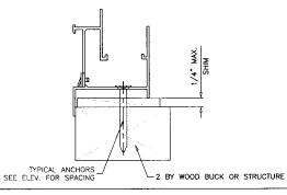
WOOD BUCKS NOT BY NUAIR, MUST SUSTAIN LOADS IMPOSED BY GLAZING SYSTEM AND TRANSFER THEM TO THE BUILDING STRUCTURE.
